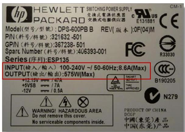
Certain IT users then assume 75% of this value for the simultaneity factor. Using the Hewlett Packard type plate shown, this would therefore mean the following:
