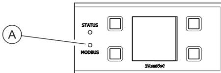
The Modbus LED (Fig. 10/Ⓐ) indicates the activity of the PDUs connected to the Modbus.
