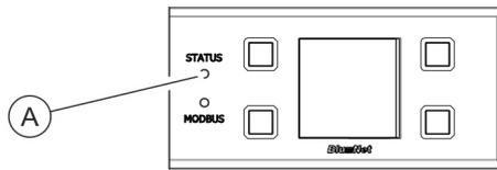
The status LED (Fig. 8/Ⓐ) indicates the status of the PDU. Possible statuses are:
