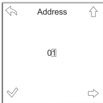
Fig. 30: Setting the Modbus address
