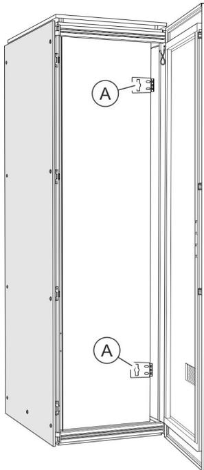
3. ➤ Remove the mounting brackets (Fig. 15/Ⓐ) from the PDU and screw them onto the rack in the positions marked.
