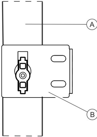
1. ➤ Fit the mounting brackets (Fig. 14/Ⓐ) onto the attachments at the top and bottom of the PDU (Fig. 14/Ⓑ).
