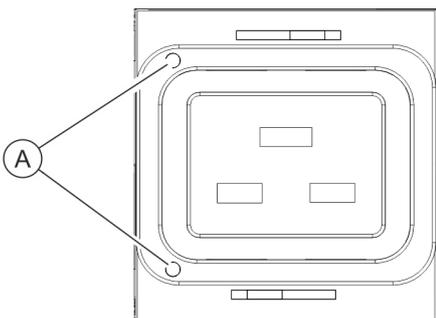
The status LEDs (only available on the BN3500/5000/7000/7500) display the status of the loads connected to the sockets.
