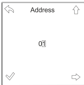
Fig. 30: Setting the Modbus address
