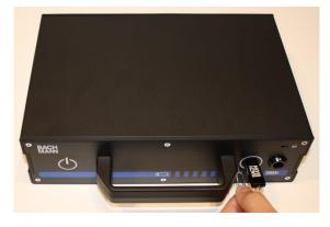
Press the reset button with the enclosed reset tool.
