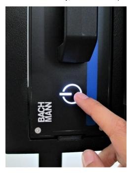
→ Press and hold the push button for approx. 2 seconds while the battery is in the docking station.
