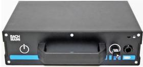
→ Plug the USB stick into the USB socket in the battery front
