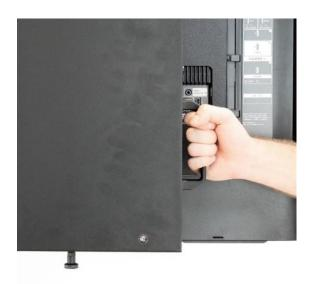
→ Hold one hand in front of the docking station so that the battery cannot fall off.
