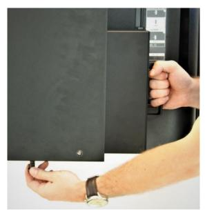
→ Push the battery completely into the docking station.
