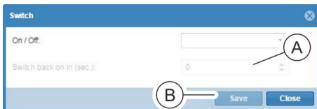
Fig. 103: Switching off a socket
