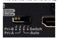
1 Switch\*: Selection of the input source via input selection button, remote control or via external control (serial control). The control LED of the selected source lights up.
