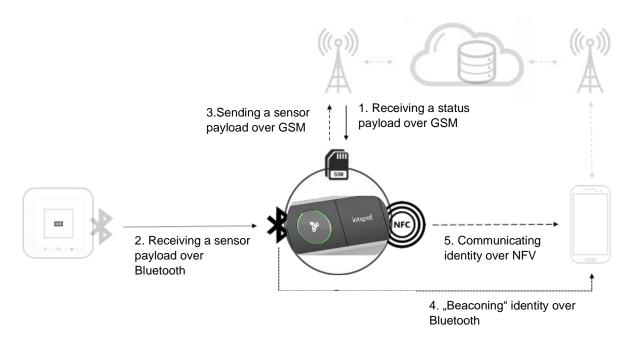
Figure 1. The iotspot module and its six functions explained.
