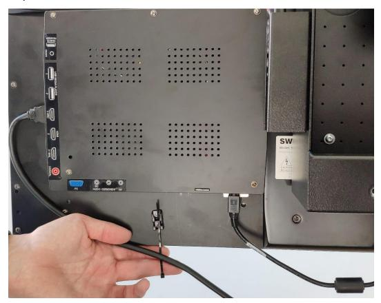
Step 14: Sort the cables and cut off cable tie.
