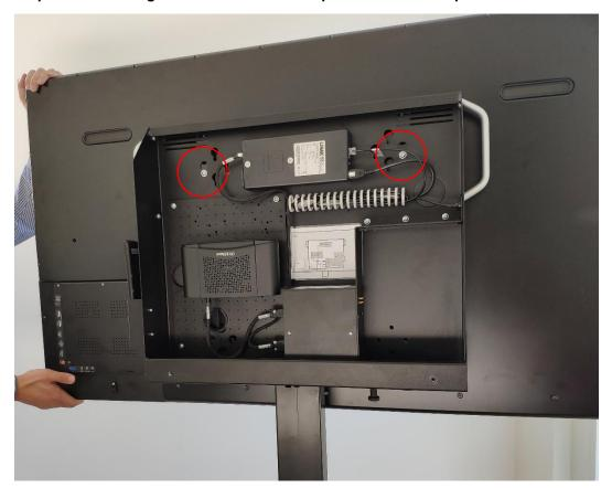
Step 7: Tighten both screws in the upper region of the monitor box.
