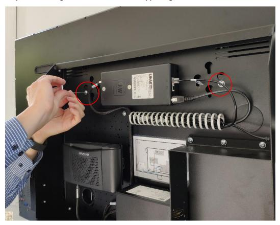
Step 8: Tighten both screws in the lower region of the monitor box.
