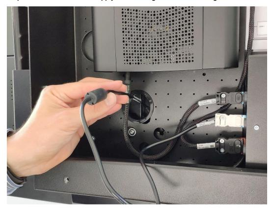
Step 11: Plug the DC supply cable into the monitor.
