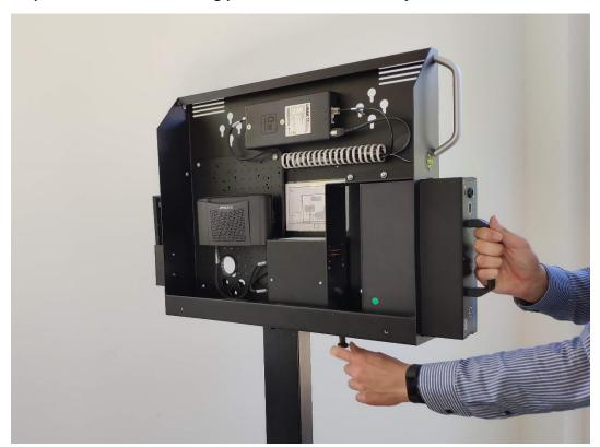
Step 6: Hang in the monitor with the pre-assembled adapter rods.
