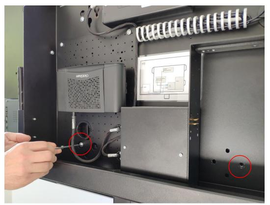
Step 9: Connect the DC supply cable (#149.0000) with the Docking Station.
