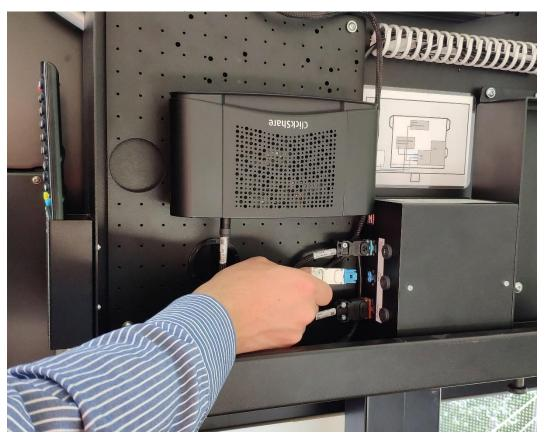
Step 10: Pass the DC supply cable through the cable bushing.
