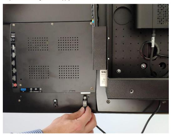
Step 12: Connect the HDMI cable to the media equipment and monitor.
